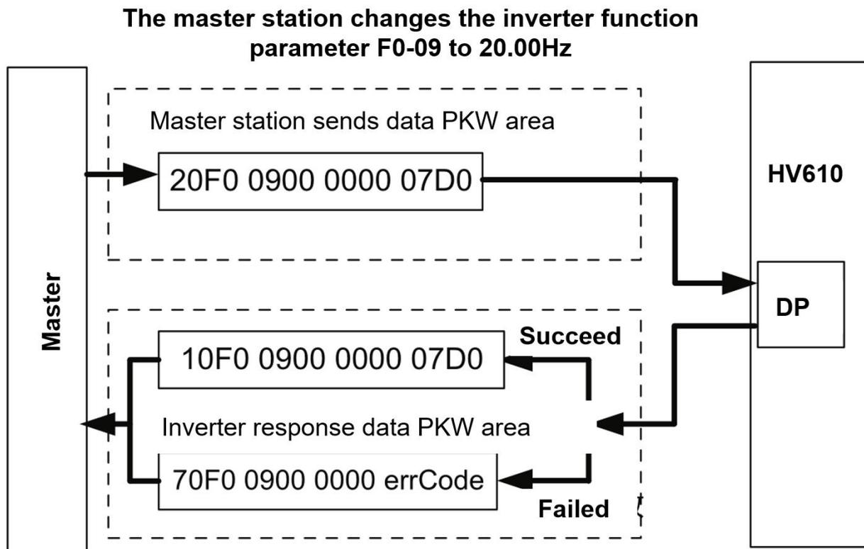
**Figure 6 Example of master station writing inverter parameters and sending PKW data**
