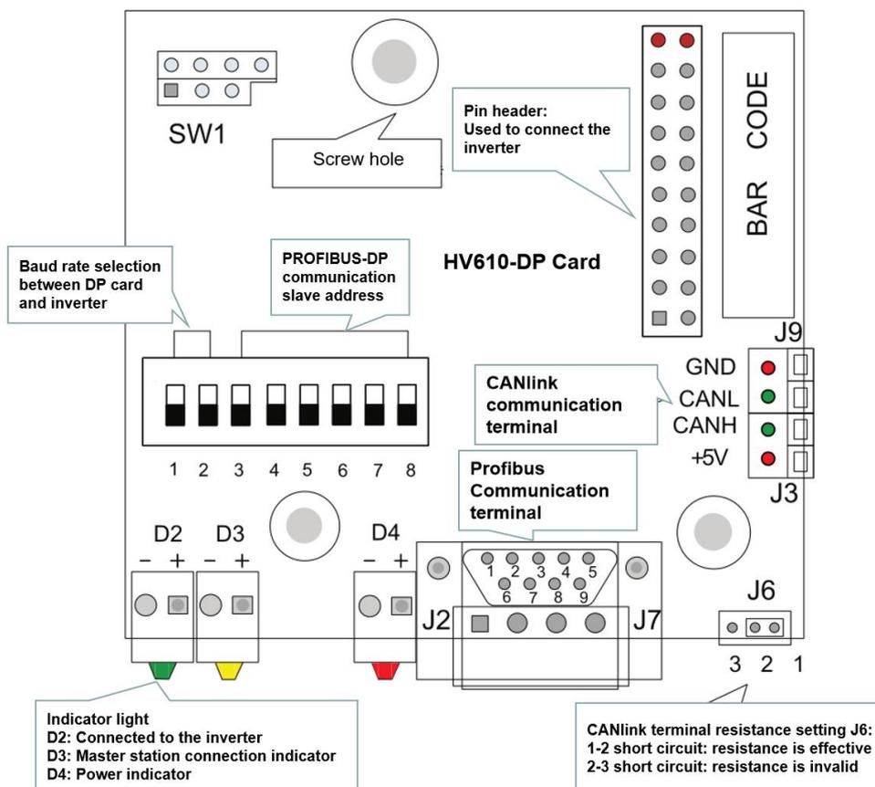
Figure 1 Terminal distribution of HV610-DP card
