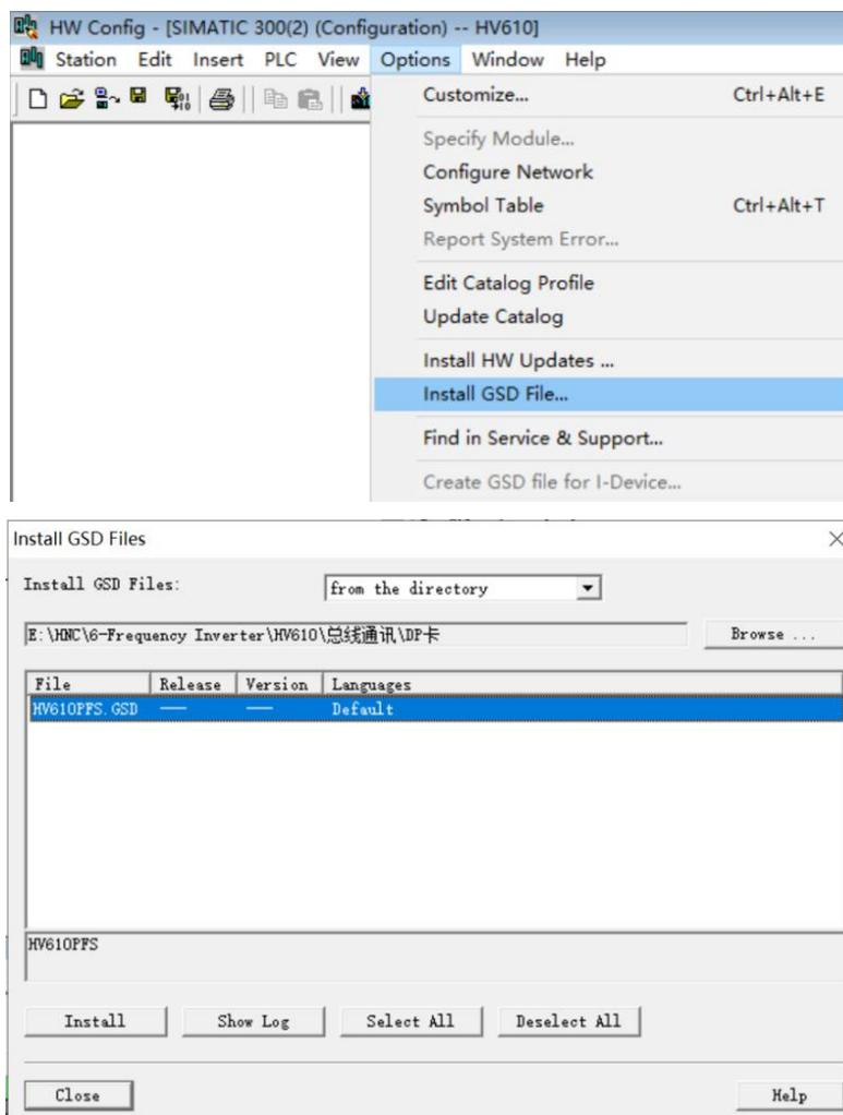
3. Click Install. After the installation is completed, there will be a PROFIBUS-DP module of MD38PFS in the system.
