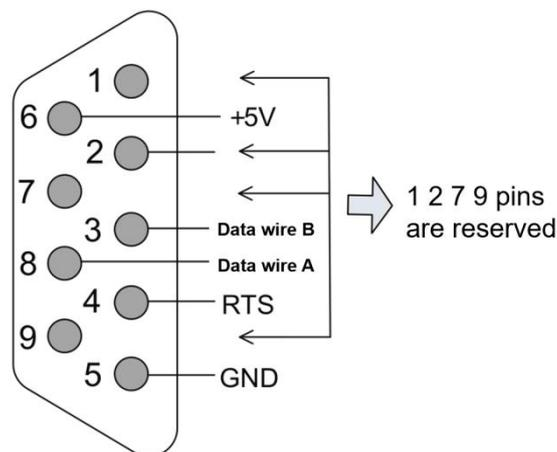
Figure 2 DB9 interface pin function description
