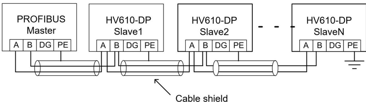
**Figure 3 Schematic diagram of the connection between the DP card and the Profibus master station**
