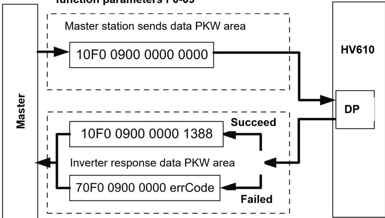
Figure 5 Example of master station reading inverter parameters and sending PKW data
